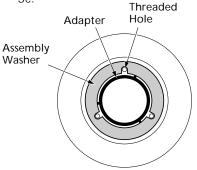
Figure 3c - Positioning Assembly Washer Slots Over Threaded Holes
